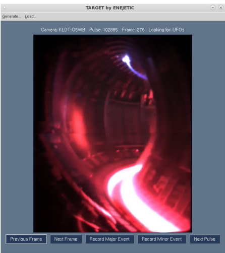
FIG. 2. The TARGET GUI, with the frame corresponding to a VSO log for pulse 102885 loaded. Users can then categorize this as either a major or minor UFO and add it to the dataset. They can then cycle through other frames in the same pulse to identify additional UFOs, before moving to the next pulse.
