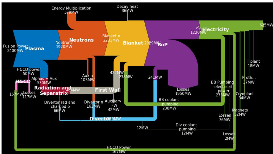
Fig. 15. Sankey diagram of an indicative pulsed DEMO power plant with  $P_{fus} = 2.4$  GW, HCPB blankets, and NBI current drive.
