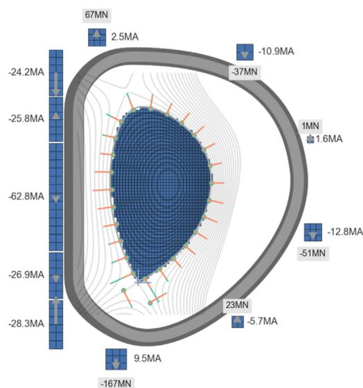
Fig. 6. Typical equilibrium solution from Nova, positioning the PF coils around the TF coils, and resulting coil currents and forces. The green and orange dots and dashes show the locations where the  $\psi$  and  $B$  values are prescribed to the optimiser.
