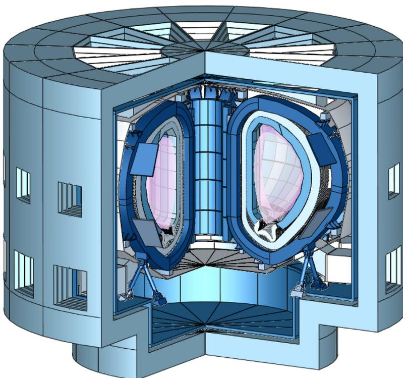
Fig. 10. Three-quarter isometric view of the 3-D CAD model of the reactor generated by BLUEPRINT in approximately 30 s, for the same design point shown in Fig. 8, with the same colour scheme. The radiation shield port plugs, cryostat vacuum vessel closure plates, and the tokamak vacuum vessel closure plates are hidden for illustrative effect.
