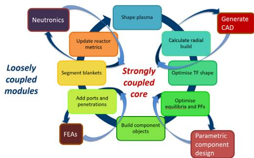
**Fig. 3.** Schematic of the BLUEPRINT design point definition approach. A tightly coupled set of calculations are performed consistent with one another. Loosely coupled procedures can generate other data upon request, but are not called in an optimisation loop.
