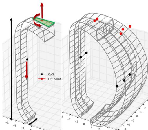
Fig. 9. Indicative plot of the important parameters required to calculate the RMTFI (segment geometries, locations of the centres of gravity, lifting locations with the port, and locations of loads and bending moments on the RM equipment).
