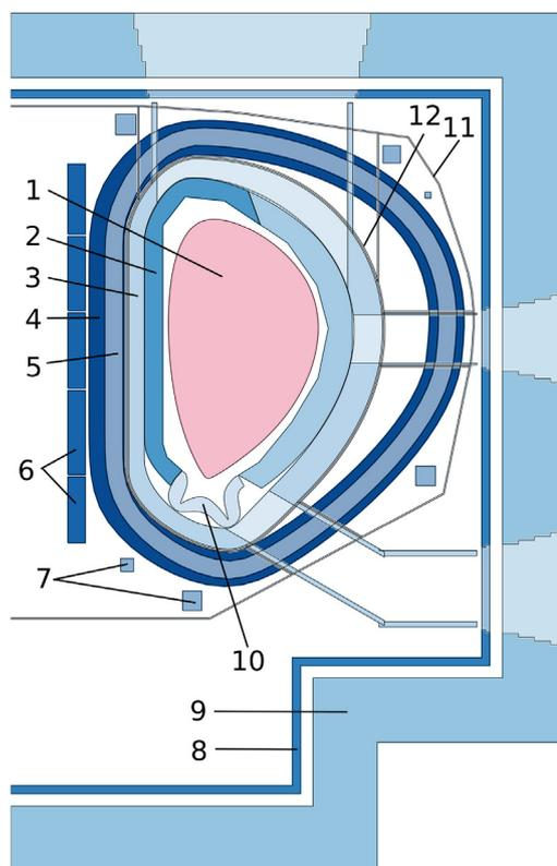
Fig. 8. Cross-section of a typical SN reactor design generated by BLUEPRINT. Legend: 1—plasma, 2—breeding blankets, 3—vacuum vessel, 4—TF coil case, 5—TF coil winding pack, 6—CS coils, 7—PF coils, 8—cryostat vacuum vessel, 9—radiation shield, 10—divertor, 11—cryostat thermal shield, 12—vacuum vessel thermal shield.
