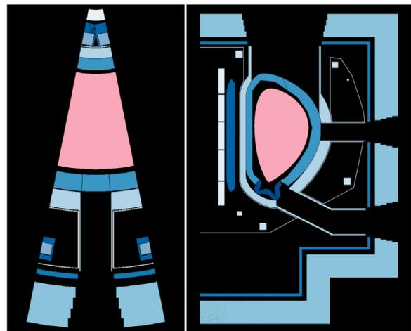
Fig. 12. Indicative Serpent II neutronics model initialised from the same reactor object as shown in Figs. 8 and 10. (left) Plan view of a sector slice at  $z = 0$ . (right) Poloidal cross-section in between two TF coils.
