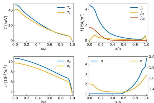
**Fig. 4.** Plasma profiles in Shafranov coordinates obtained using the PLASM0D code, showing (clockwise) the electron and ion temperature ( $T_e$  and  $T_i$ ), the parallel, bootstrap, and driven currents ( $j_{||}$ ,  $j_{bs}$ , and  $j_{CD}$ ), the electron and ion densities ( $n_e$  and  $n_i$ ), and the safety factor,  $q$ , and elongation,  $\kappa$ , profiles.
