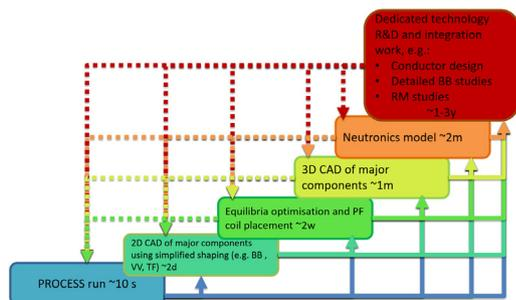
Fig. 2. Schematic representation of the DEMO reactor design point definition and evaluation procedure in Europe.
