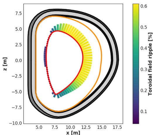
Fig. 5. Plot of the toroidal field ripple on the separatrix (shown in red) for an optimised “S” TF coil, with  $n_{TF} = 16$ . The TF coil exclusion zone constraint (VVTS outer surface) is plotted in orange.
