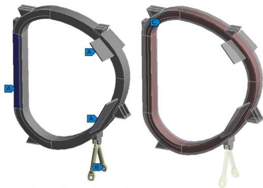
Fig. 11. Indicative ANSYS TF FE model. Showing boundary conditions: (A) cyclic symmetry; (B) frictionless support, and sliding friction joint condition between the WP and the TF coil casing (C). NOTE: The gravity supports shown here are inspired from the JT60-SA design, and have not been designed or analysed. The intercoil structures are similarly indicative; indeed this coil would likely fail under the combined loads in its present form.
