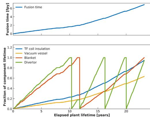
**Fig. 13.** Example of a DEMO-class reactor lifecycle generated by BLUEPRINT. Above the evolution of the reactor fpy over its life is shown, and below is the build-up of damage in key reactor components throughout the course of operation of the reactor.
