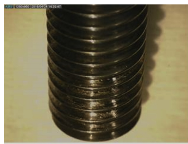
Fig. 9. MoST Coating Damage After 6 Cycles.
