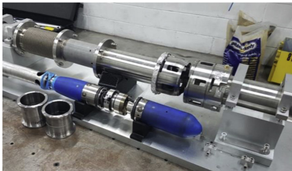
Fig. 6. Weld tool and welded P91 and 316 L samples.
