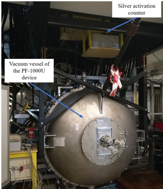
Fig. 1. Image of the PF-1000U device vacuum vessel also showing the G-M tube-based silver activation diagnostic position, described in detail in [3].
