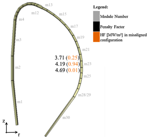
Fig. 3. Penalty factor poloidal map for \pm 10 mm misalignment during RU. Only penalty factors greater than 1 are shown.
