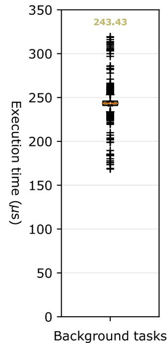
Fig. 5. Background activities in the real-time threads usually use around 250  $\mu\text{s}$  in each cycle.
