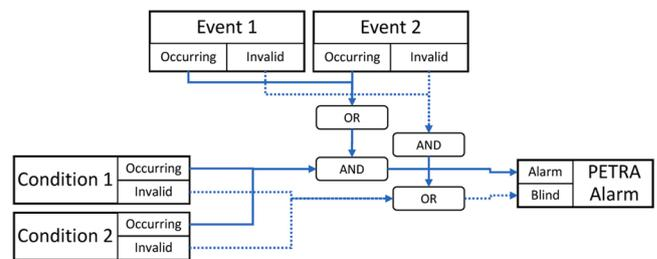
Fig. 1. Each PETRA alarm and blind is a logical combination of the connected events and conditions.
