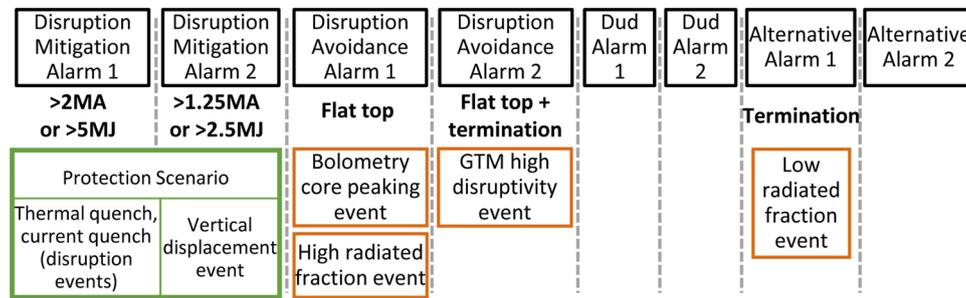
Fig. 3. A typical pulse allocates event detectors to the various PETRA alarms to target different exceptions in different phases of the plasma.
