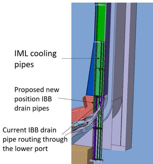
Fig. 13. Vertical pipe chute.
