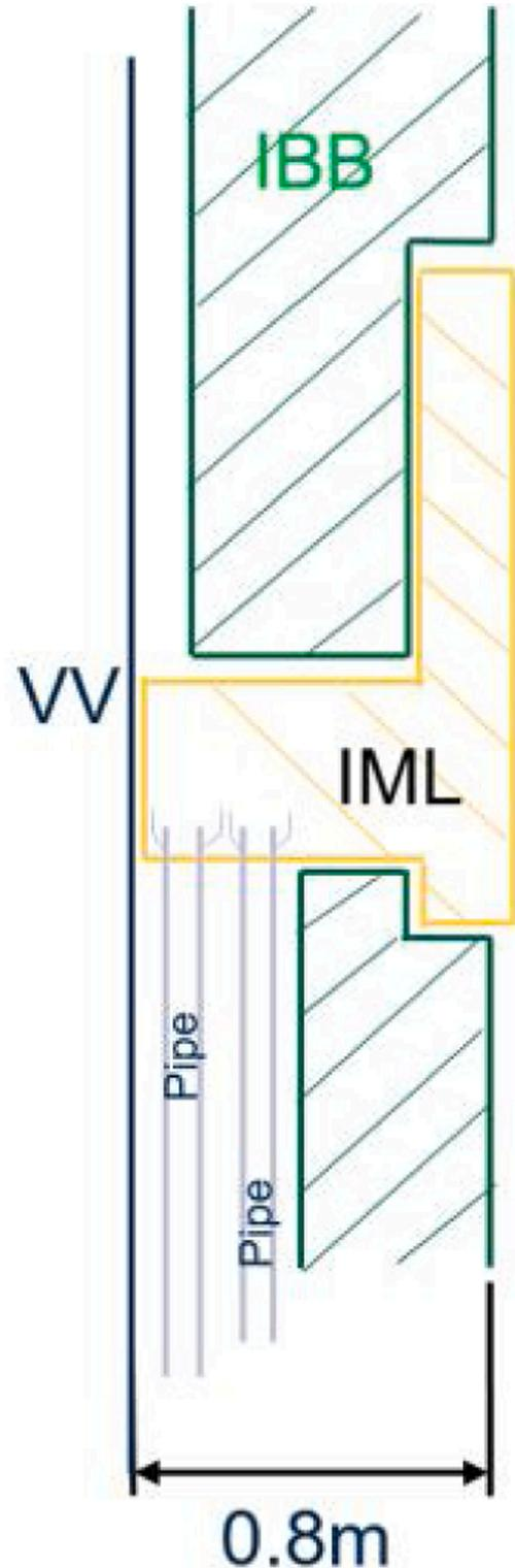
Fig. 8. Concept C - Blanket mounted limiter (section view from side).
