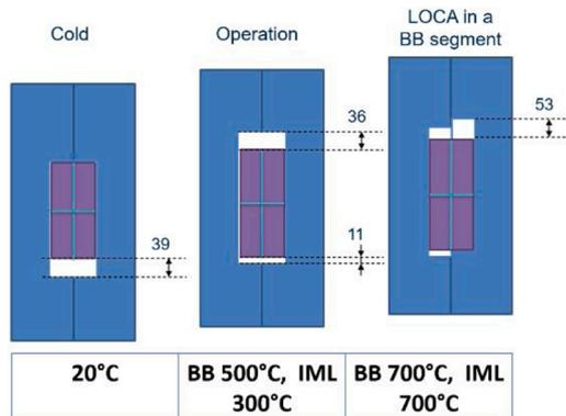
Fig. 3. IML and BB varying clearances with temperature (view towards the tokamak centre).
