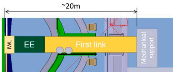
Fig. 2. Diagram showing the IML and the intended maintenance equipment approach through the equatorial port.
