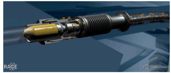
Fig. 4. DEMO in-bore laser welding tool.
