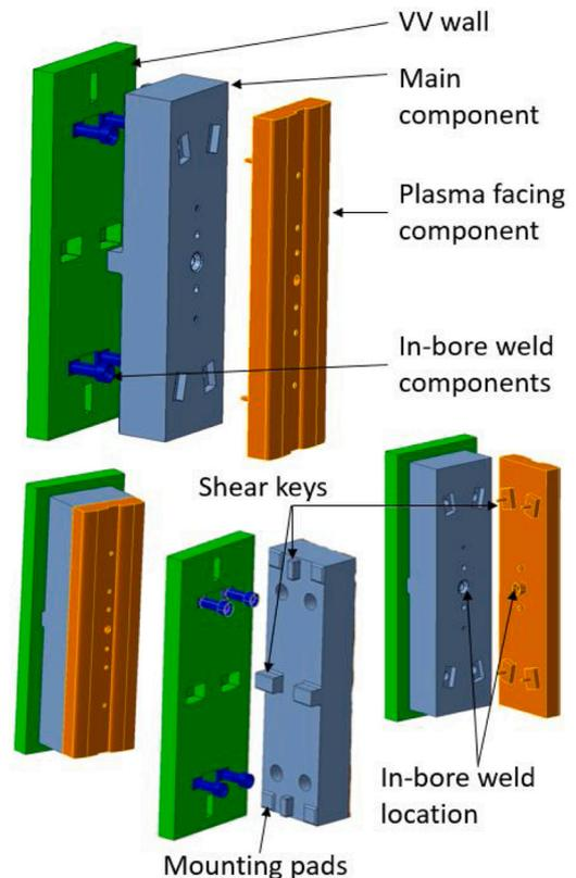
Fig. 5. Concept A – Two-piece limiter.
