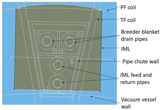
Fig. 11. Vertical pipe chute sketch – bottom view (with a toroidal cross-section).
