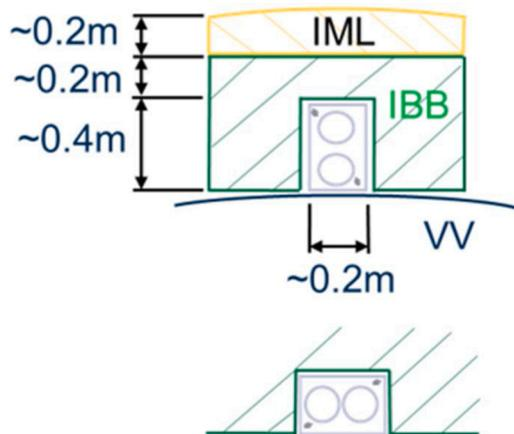
Fig. 7. Concept C - Blanket mounted limiter (section view from underneath. Alternative pipe arrangement shown).
