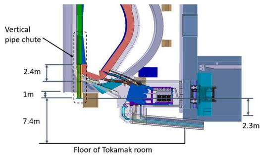
Fig. 12. Tokamak side view with vertical pipe chute.
