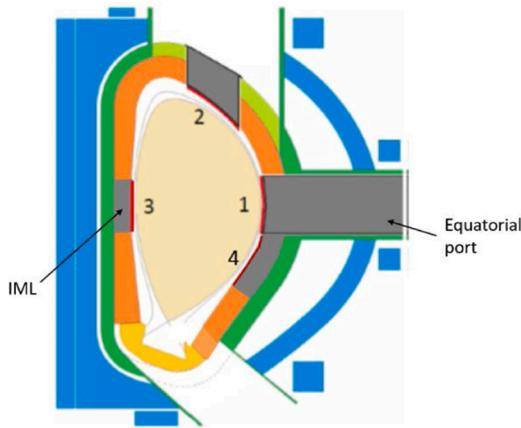
Fig. 1. Schematic view of the Single Null EU DEMO indicating the positions which the limiters occupy [2].
