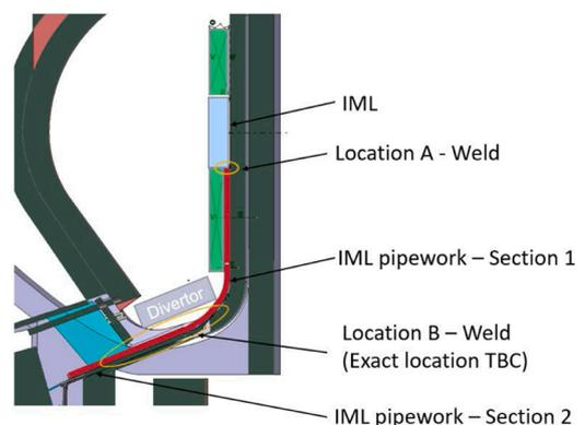
Fig. 10. Multi-piece limiter pipework.
