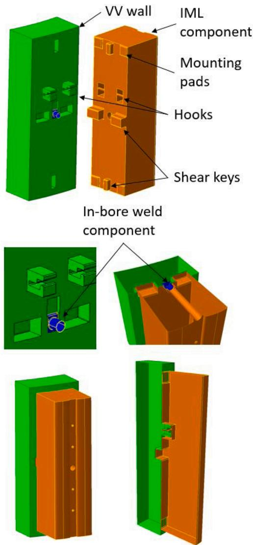
Fig. 6. Concept B Single piece limiter.
