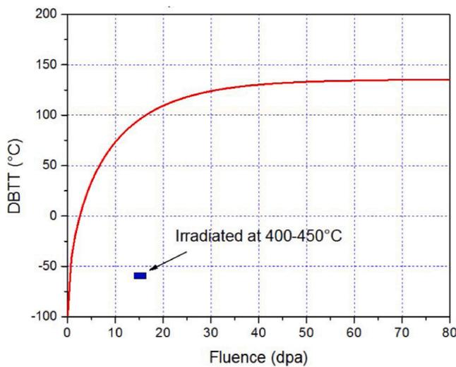
Fig. 2. show the change in Ductile to Brittle Transition Temperature (DBTT) of EUROFER97 as a function of the fission neutron irradiation fluence (dpa) obtained on KLST specimens irradiated at 250–340 °C. The blue point (rectangle) represents KLST specimens after fission neutron irradiation but irradiated at 400–450 °C [20]. (For interpretation of the references to colour in this figure legend, the reader is referred to the web version of this article).
