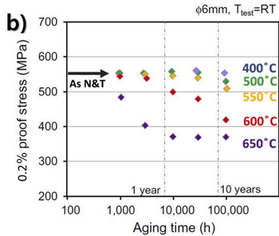
Fig. 1. a) creep life for various RAFM and Grade 91 steels at various temperatures, b) yield strength vs aging time for F82H RAFM steel at various ageing temperatures [21,24,25].
