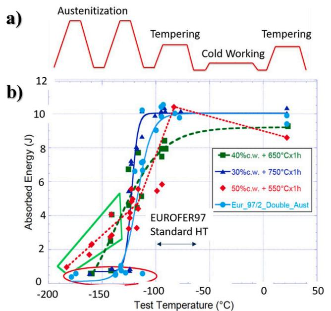
Fig. 4. a) example of a new thermodynamical processing procedure for EUROFER, b) absorbed energy vs test temperatures for new variations of EUROFER that underwent new thermo-dynamical processing conditions showing reduced transition temperatures compared to that of conventional/standard EUROFER97 [37–39].
