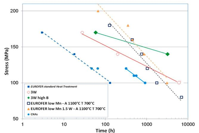
Fig. 5. variation in stress rupture times for various “modified” EUROFER steels, with conventional/standard EUROFER97 included for reference [40,41].
