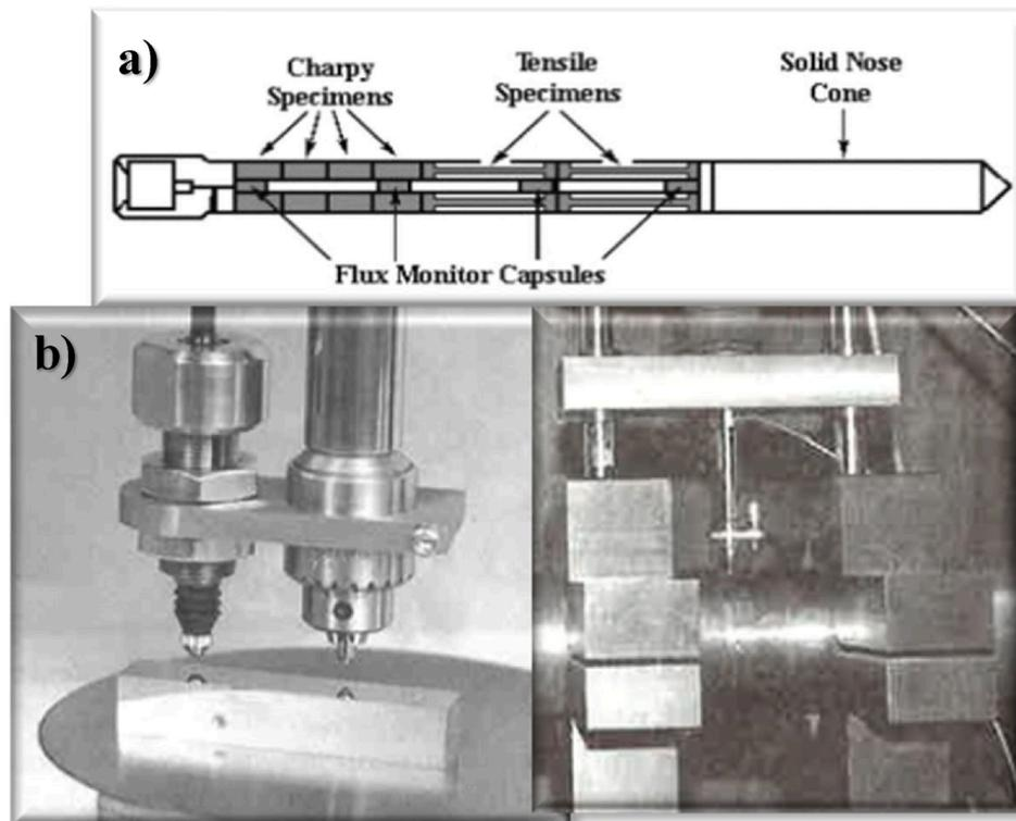
Fig. 3. a) example of surveillance cell use in fission reactors, b) left, example of hardness profile testing technique and right, example of the same testing technique used in-situ on a pipe [33,34].
