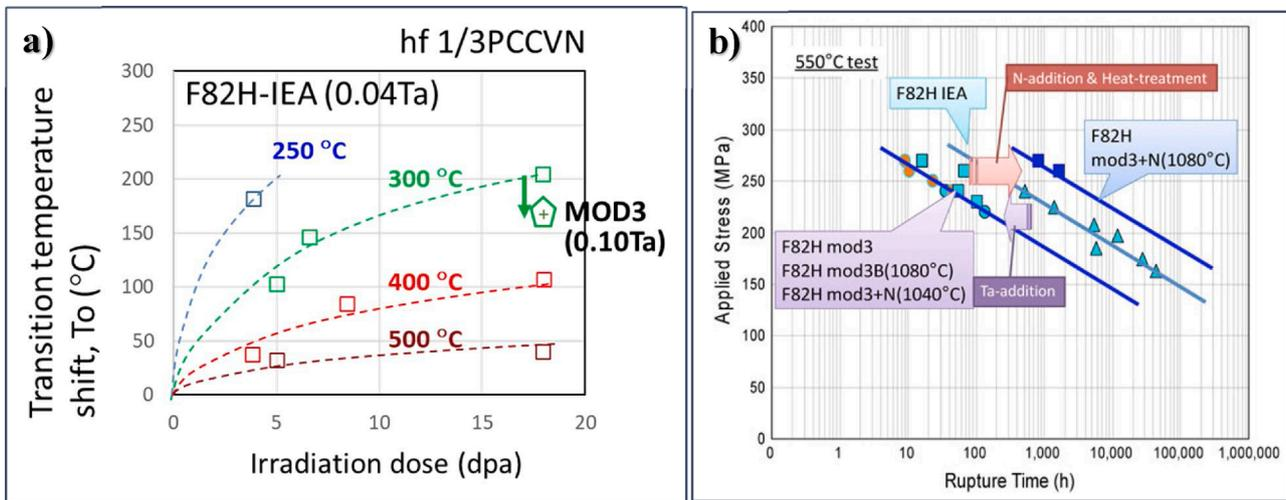
Fig. 6. a) transition temperature shifts vs irradiation dose (dpa) for F82H-IEA and example of shift due to modifications MOD3, with increased Ta content. B) creep strength of various F82H alloys following modifications to conventional/standard F82H IEA grade [42–45].
