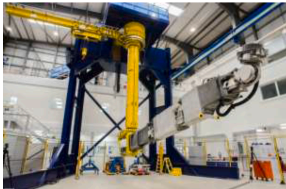
Fig. 28. Refurbished TARM installed on a bespoke remote maintenance testing stillage at UKAEA.
