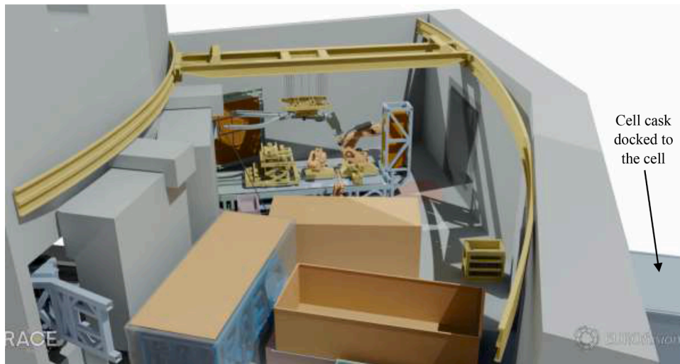
Fig. 19. Image of the large port cell approach for maintenance of the lower port
