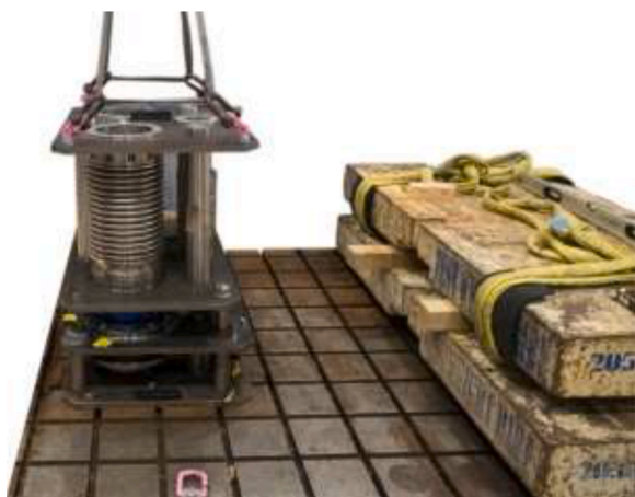
Fig. 27. Passive alignment mechanism testing showing pipe module dead-weight simulant at right
