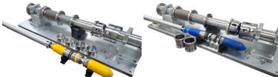
Fig. 22. Laser cutting tool (left) and welding tool (right) both with samples in P91 and 316L
