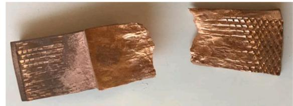
Fig. 20. Sheared CuCrZr-Cu specimen brazed with OB1025™.
