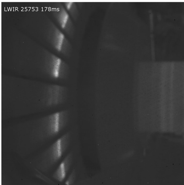
Fig. 7. Some of the tiles in the divertor of MAST during shot 25735. The tile in the centre of the image had just been replaced, and the strike point is very faint on this tile compared to the others.
