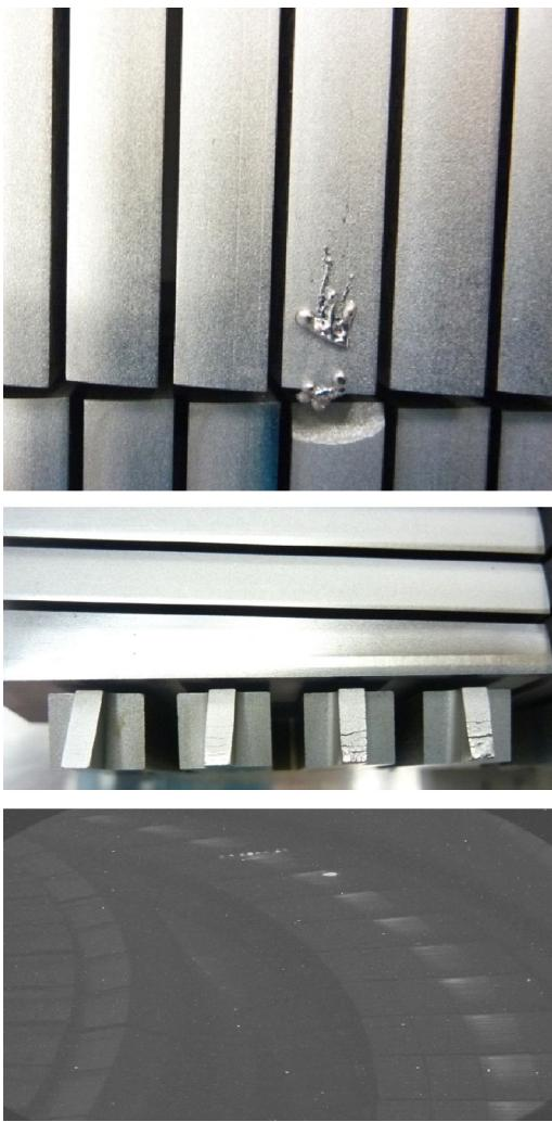
**Fig. 5.** Collection of tungsten melts: (top) inboard edge of one lamella on the outermost stack; (middle) Langmuir probe tips melted and cracked; filtered visible camera view showing one set of Langmuir probes (top chain of dots) and the lamella melt of the top picture (large isolated hot spot).
