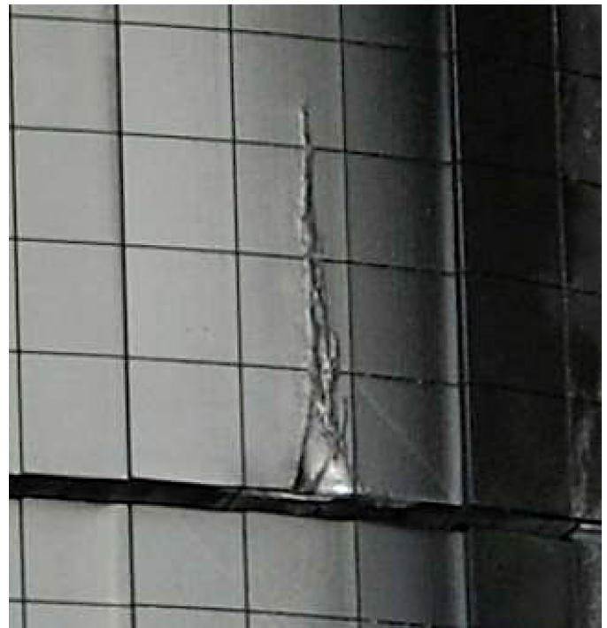
**Fig. 6.** Langmuir probe on the inner wall guard limiter and damage on the neighboring beryllium tile.
