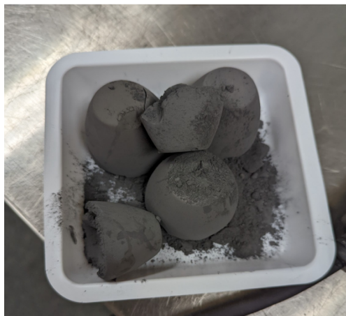
Figure 4.32: Powder cake W-28Cr at% powder for SPS in cake form.
