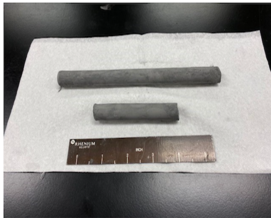
Figure 4.14: CIPped W-28Cr at% bars 2 bars of W-28Cr at% after slow CIPping and prior to the pre-sintering phase.
