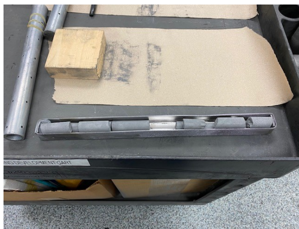
(a) W30Cr (wt.%) after slow ramped pre-sintering phase.
