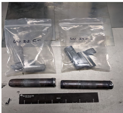
Figure 4.18: Sintered bars of W-28Cr at% alloy W-28Cr at% samples after sintering in molybdenum cans for 8 hours at 2000 °C
