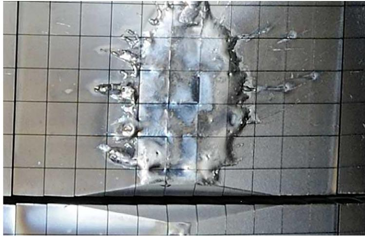
**Fig. 4** A photograph of a re-solidified area of a beryllium plasma-facing component in the JET tokamak following a melting event. Matthews GF, et al. (2016) Melt damage to the JET ITER-like wall and divertor. *Physica Scripta* T167: 14070. doi: 10.1088/0031-8949/t167/1/014070.
