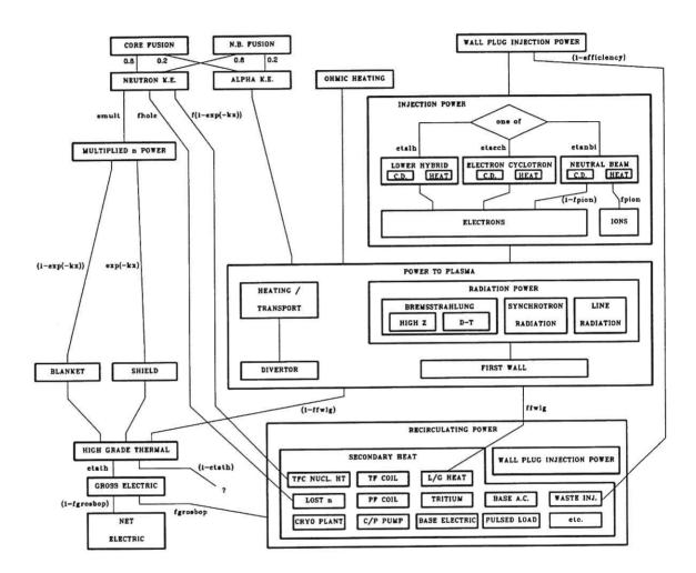
Figure 2.5: Schematic diagram showing the power conversion mechanisms used in PROCESS [15, Note 0166].
