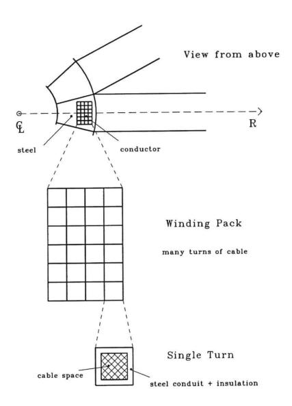
Figure 2.3: Schematic diagram of the cross-section of a superconducting TF coil, showing the CICC (Conductor In Cable Conduit) construction. The cable space contains superconducting filaments and circulating liquid helium coolant.
