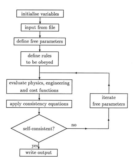
Figure 2.6: Flow diagram of PROCESS in non-optimisation mode.
