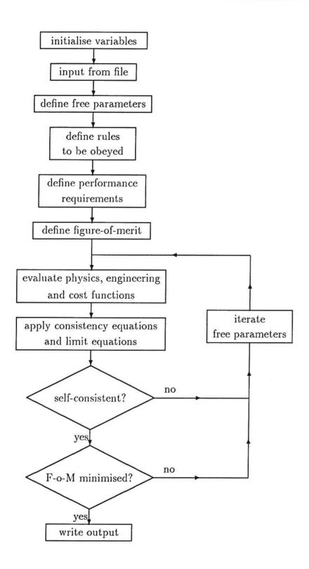
Figure 2.7: Flow diagram of PROCESS in optimisation mode.
