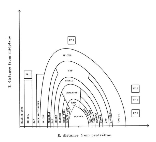
Figure 2.1: Schematic diagram of a typical tokamak modelled by PROCESS. The relative positions of the components are as shown, assuming that switch iohcie is set to 2. If iohcie is set to 1, the inboard portion of the radial build is altered so that, starting at the centreline (R=0), the component order is: bucking cylinder, TF coil, gap, OH coil, cryostat, etc. In this case there is no machine bore. The numbers shown in the PF coil blocks are the values of the ipfloc switch for that block.
