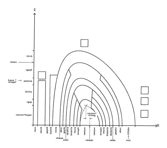
Figure 2.2: Schematic diagram of a typical tokamak modelled by PROCESS, showing the variables used to define the thicknesses of the components. The arrowed labels adjacent to the axes are the total 'builds' to that point. As in Figure 2.1, the relative positions are shown for the case when iohcie = 2. The precise locations and sizes of the PF coils are calculated within the code.
