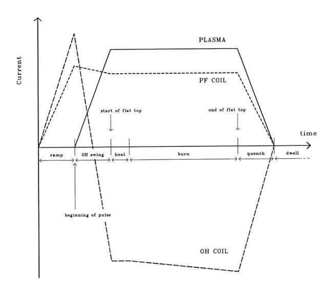
Figure 2.4: Plot showing schematically the current waveforms for the plasma, a typical PF coil, and the OH coil.
