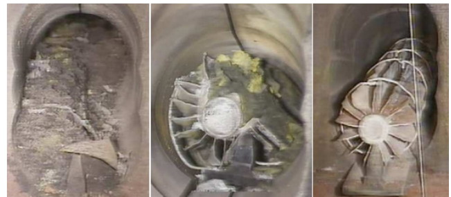
Fig. 2. Fuel element conditions in pile 1: destroyed, severely damaged, and with minor damage around the fire affected zone [10].
