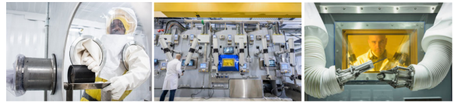
Fig. 6. Gloveboxes where the operator is wearing special gloves for protection while analysing/examining hazardous material or using local-remote robotic manipulator system for the enhanced safety measures. Sources: U.S. Department of Energy and UKAEA.
