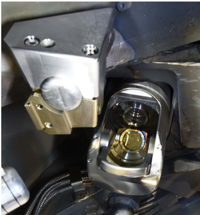
Figure 3. Mirror protection clamp installed on the crane rail boss (top left), the gold coated periscope mirror is undamaged after a year of plasma operation (picture was taken in February 2017).
