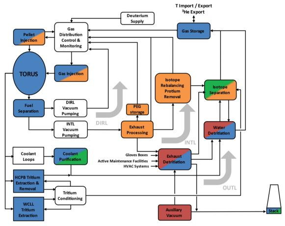
Fig. 1. Diagram of subsystems in the fuel cycle,<sup>2</sup> with colors indicating for which purpose tritium measurements need to take place. Blue: nonproliferation; green: environment; red: safety; orange: plasma composition control. General process control measurements can be expected to take place in almost every location and are hence not displayed here.
