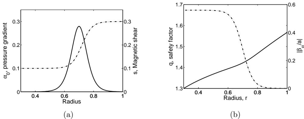
Figure 3: Transport barrier profiles used in this numerical investigation: a) magnetic shear,  $s(r)$ , and pressure gradient  $\alpha(r)$ ; and b) safety factor and pressure profiles used for this numerical investigation.
