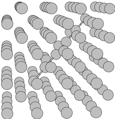
FIG. 1: Atomic structure of a self-interstitial atom defect in tungsten, where the orientation of the axis of the defect is close to the  $[111]$  direction. Atomic bonds are shown for the atoms that are significantly closer to each other than atoms in a perfect lattice.
