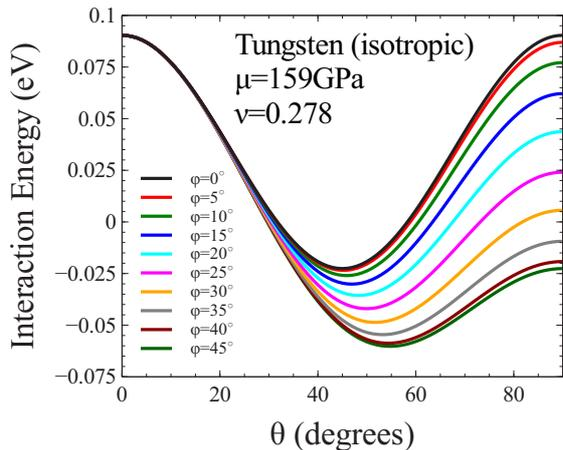
FIG. 4: (Color online) Energy of elastic interaction between a  $\langle 111 \rangle$  self-interstitial atom defect and its images in tungsten as a function of the orientation of vector  $\mathbf{n}$ , computed using data from Table V in the isotropic elasticity approximation.
