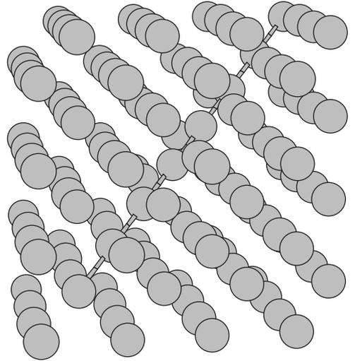
FIG. 2: Atomic structure of a self-interstitial atom defect in vanadium, where the orientation of the axis of the defect is close to the  $[111]$  direction. Atomic bonds are shown for the atoms that are significantly closer to each other than atoms in a perfect lattice, similarly to the case of tungsten illustrated in Fig. 1. Note that the strain field of a defect in vanadium is less localised than the strain field of tungsten.
