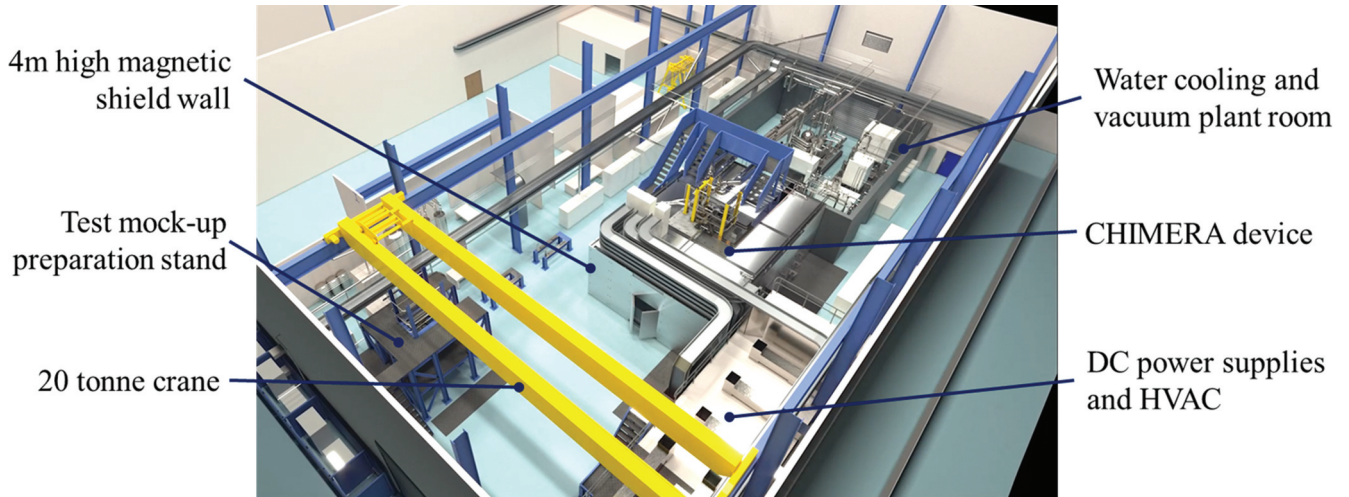
Fig. 1. Aerial isometric view (computer-aided design) above the CHIMERA facility.
