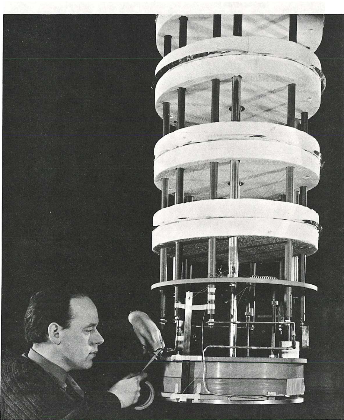
Fig.4 Pair of 425mm coils being assembled for test. CLM-P 238
