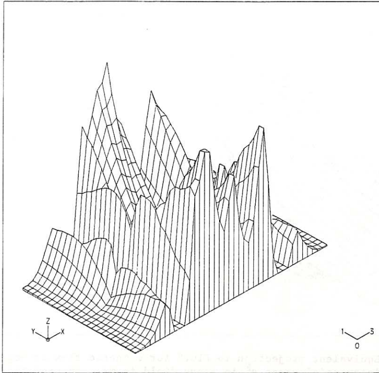
FIG. 7 Equivalent projection to FIG.3 for cell volumes V . Very small values adjacent to targets reflect clustering of grid both in facing high recycling regions and around separatrix.
