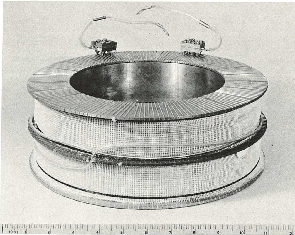
Fig. 2 30 kG 8½ inch bore superconducting coil (CLM-P 90)
