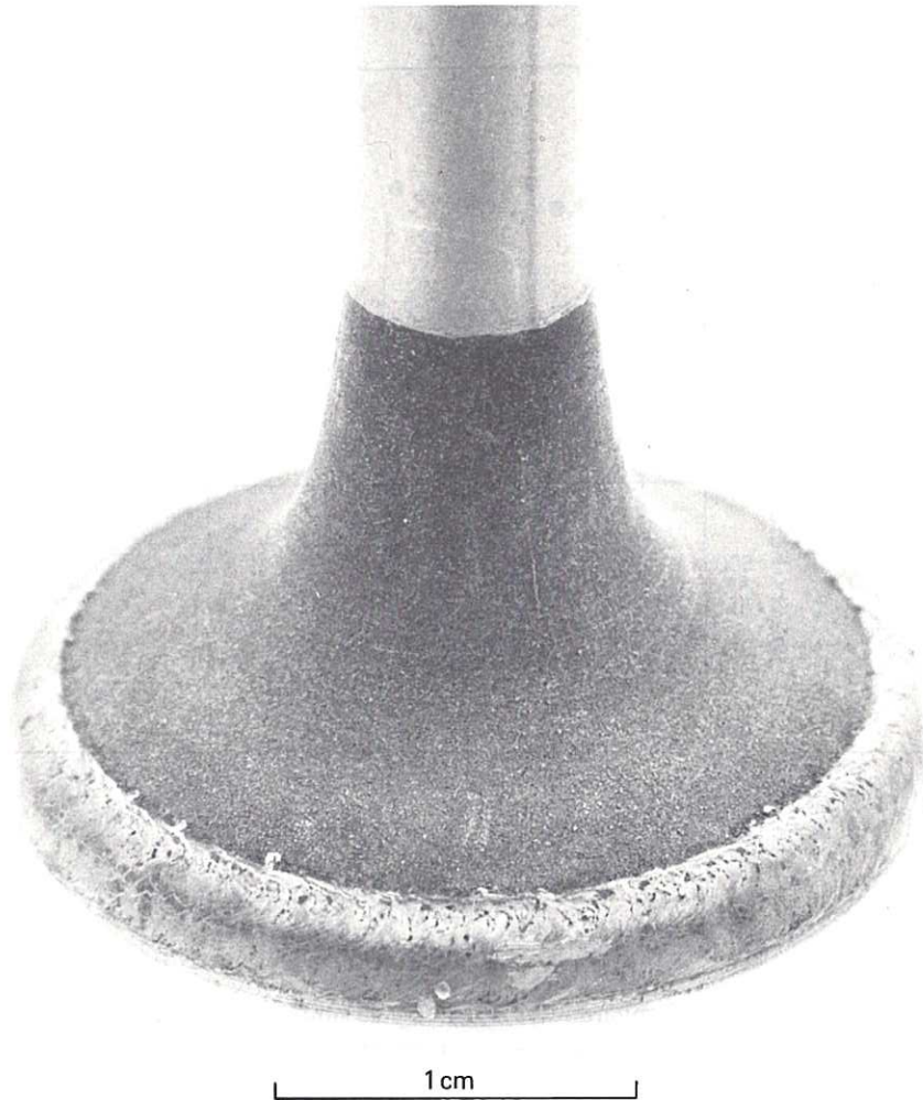
Fig.7 Car engine exhaust valve with Stellite facing on seat deposited by 4.5kW laser beam.
