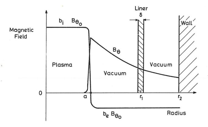
Fig. 1 Equilibrium field configuration showing edge of plasma, liner and conducting wall.
