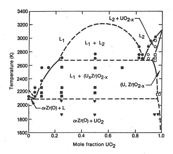
Figure I Oxygen Stabilised, Alpha Phase Zirconium-Uranium
