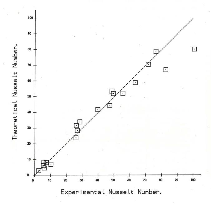
Figure 3 Comparison of Theoretical and Experimental Nusselt Numbers for the Density Stratified Study of Kulacki and Nguyen.
