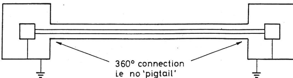
Fig. 6.7: Optimum cable screening, no pigtails.
