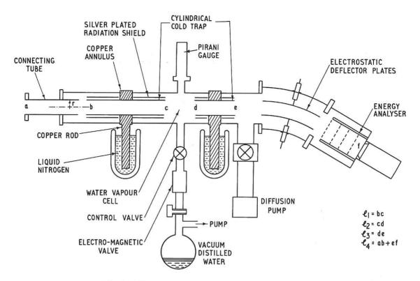
Fig.1 Fast atom detector (schematic) (CLM-R49)
