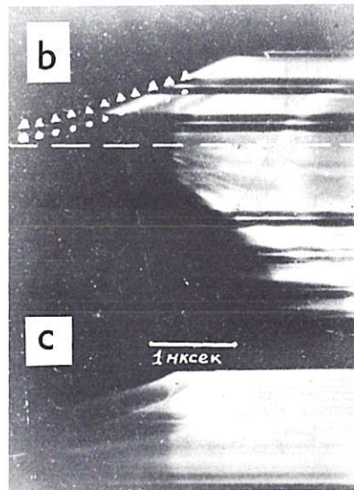
Fig. 2(b) & 2(c) (CLM Trans 8) Streak photographs taken: b - through slit II ; c - through slit III ; dotted line - electrode limit; dots - radial displacement of envelope away from insulator calculated from (4) and (6); triangles - boundary of the skin-layer, calculated from (1)
