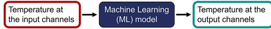
FIG. 11: Outline of the ML model used for the transient thermal field reconstruction. The temperature values at the six input channels are given to the ML model, whereas the temperature values at the 194 output channels are generated by the ML model. The locations of the six input channels are randomly selected.
