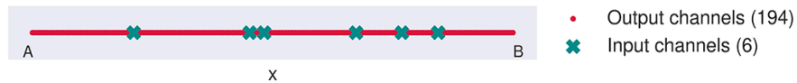
FIG. 9: The 1-D grid used to generate the GT for 1-D transient heat conduction. The input and output channels of the mesh nodes are highlighted, with the six green crosses being the input channels and the 194 red dots being the output channels. The temperature values at the six input channels are given to the ML model, whereas the temperature values at the 194 output channels are generated by the ML model at every time step, which is equal to 1s in this case. The locations of the six input channels are randomly selected.
