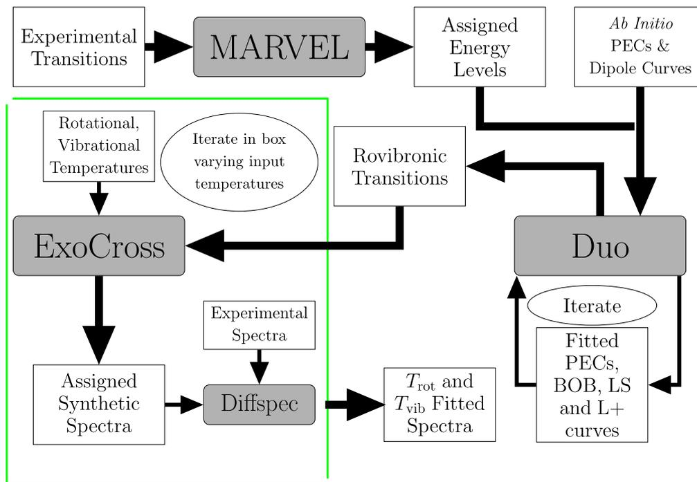
**Figure 1.** Flow diagram showing the production of high accuracy synthetic spectra, starting in the top left corner with collated experimental transitions and resulting in, bottom center, synthetic spectra with the best fit rotational and vibrational temperatures.
