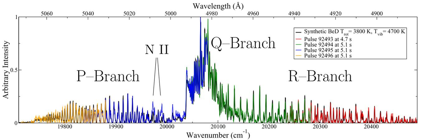
**Figure 5.** Measured BeD spectra, in red, green, blue and orange lines with pulse numbers and times in the legend, were recorded with a high resolution spectrometer,  $T_e \approx 30$  eV and  $n_e \approx 10^{-18}$  m $^{-3}$ . Assigned synthetic spectrum, in black, is generated with  $T_{\text{rot}} = 3800$  K and  $T_{\text{vib}} = 4700$  K using our BeD line list.
