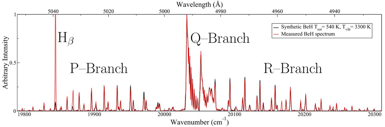
**Figure 4.** Measured BeH spectrum, shown in red, was recorded with a high resolution visible spectrometer from a hydrogen doped lamp with a beryllium target. Assigned synthetic spectrum of BeH, in black, is generated with  $T_{\text{rot}} = 540$  K and  $T_{\text{vib}} = 3300$  K using our BeH line list.
