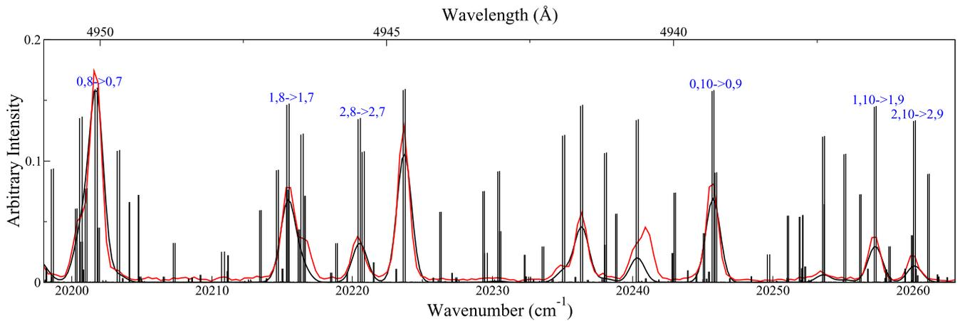
**Figure 6.** Magnified R-branch synthetic BeH A–X spectrum as in figure 4, generated at  $T_{\text{rot}} = 540$  K and  $T_{\text{vib}} = 3300$  K. Measured BeH spectrum is shown in red and transition assignments with drop lines in black. Assignments show in order left to right:  $v'' =$  upper state vibrational quantum number,  $N'' =$  upper state nuclear rotational quantum number,  $v' =$  lower state vibrational quantum number,  $N' =$  lower state nuclear rotational quantum number.
