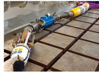
Fig. 2.2. Cutting/Welding Tool on deployment system.
