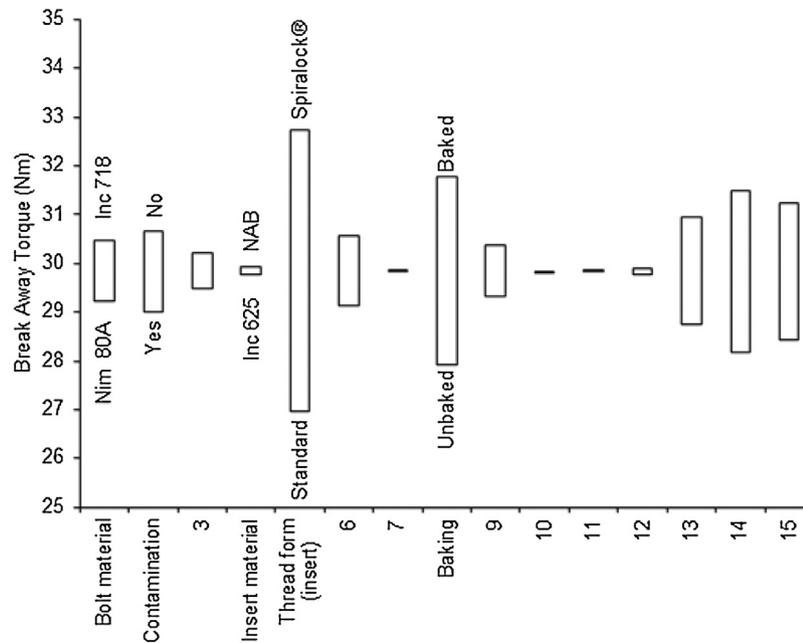
Fig. 7. Breakaway Torque Response – Effects Plot.
