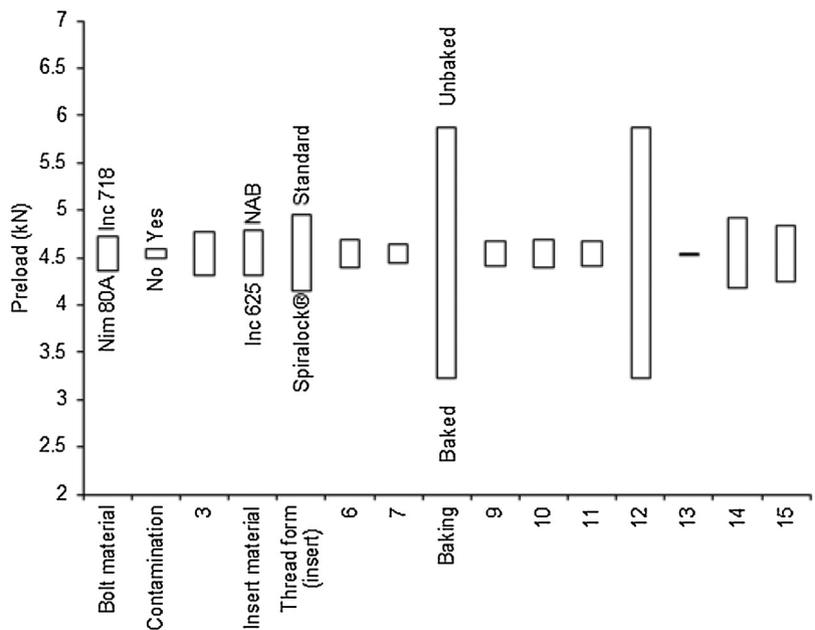
Fig. 6. Bolt Preload Response Effects Plot.
