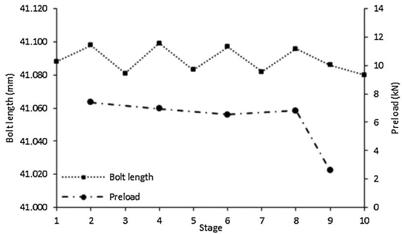
Fig. 5. Sample Bolt Length and Preload Data.
