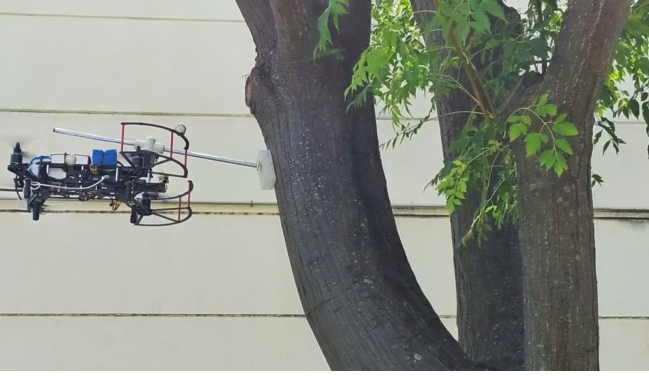
Fig. 3: Direct sensor placement on a tree with an aerial robot.
