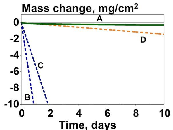
**Fig. 2.** Mass reduction due to sublimation as a function of exposure time for W-Cr-Y smart alloy (curve A), fully oxidized tungsten thin film (curve B), oxidized bulk W sample (curve C) and for oxidized pure Cr film (curve D) in humid air at 1000 °C.
