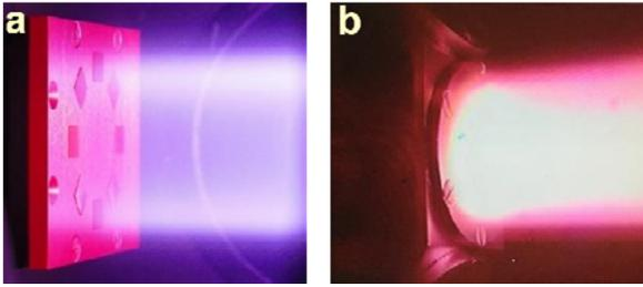
**Fig. 1.** Photographs of plasma exposures in linear devices: a) simultaneous exposure of smart alloy and pure tungsten samples in linear device PSI-2 and b) consecutive one-by-one exposure in MAGNUM PSI.
