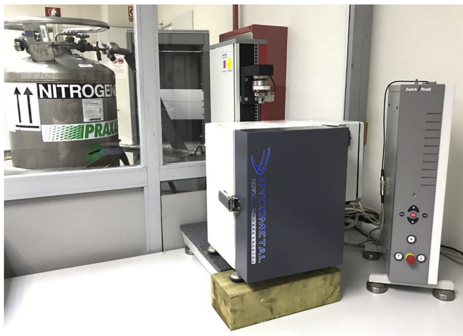
Fig. 1. Environmental chamber and testing rig employed for the performance of the small punch tests.
