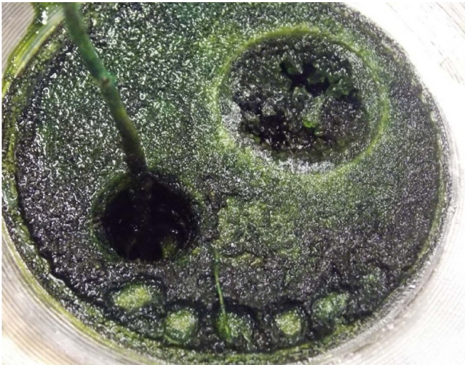
Figure 19. Green residue build-up on bottom flange following chronic HCl testing of Verdal.
