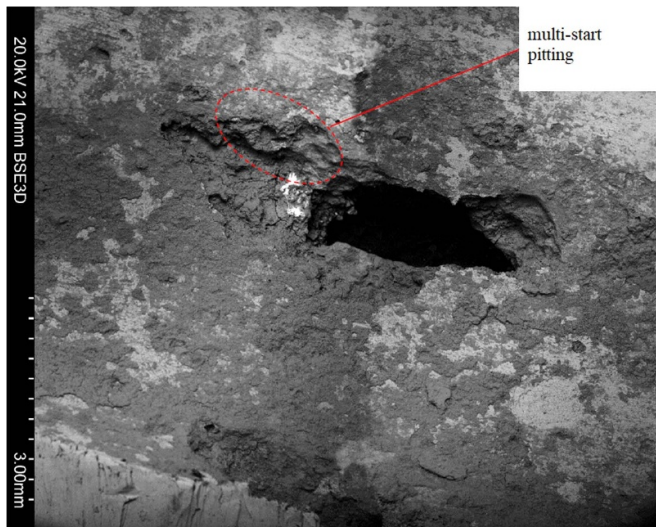
Figure 5. Scanning electron micrograph of perforation (location of pipe failure).
