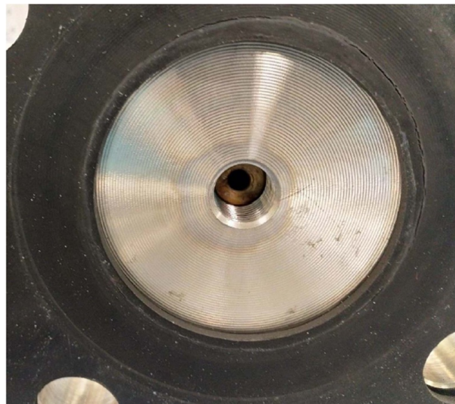
Figure 17. Light pitting corrosion on outlet flange during acute HF testing Intersorb.
