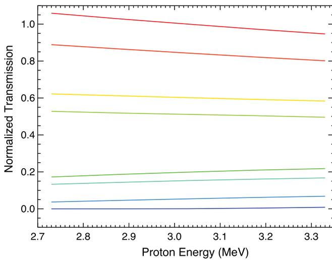
**Figure 4.** The overall transmission of the collimator increases with energy because the incident orbits are straighter. A variety of different incident velocity vectors are shown. The curves are normalized to the transmission of the maximum velocity vector for  $E_3 = 3.03$  MeV.
