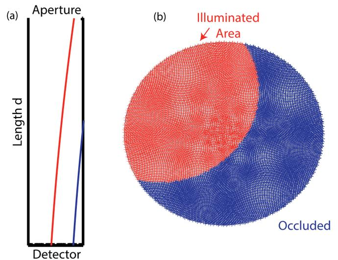
**Figure 2.** (a) Schematic diagram of a cylindrical collimator. For a given orientation of the incident proton velocity, some orbits reach the detector (red), while others do not (blue). (b) For a given incident velocity vector, only the red portion of the detector is illuminated. The figure also shows the sunflower sampling of the detector area.
