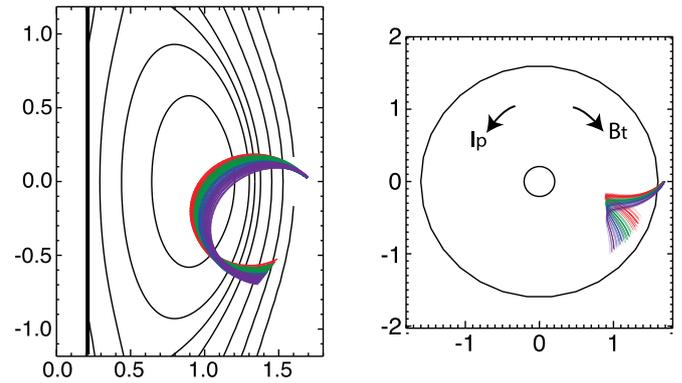
**Figure 1.** Elevation (left) and plan (right) views of 3.03 MeV proton orbits (colors) that reach the four MAST proton detectors in a particular equilibrium. The thickness of the lines is proportional to the effective transmission  $T$ . The black lines in the elevation represent flux surfaces (thin lines) and the inner wall of the vacuum vessel (thick line). The directions of plasma current  $I_p$  and toroidal field  $B_T$  are also indicated.
