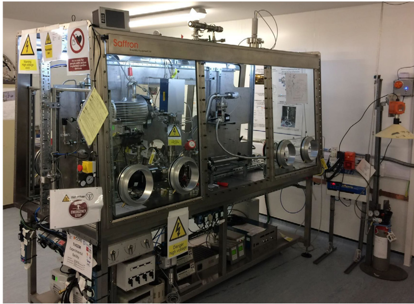
Figure 1. Plasma exposure system after inactive gas commissioning. The system is partially built into the secondary containment system which will be required for tritium commissioning.
