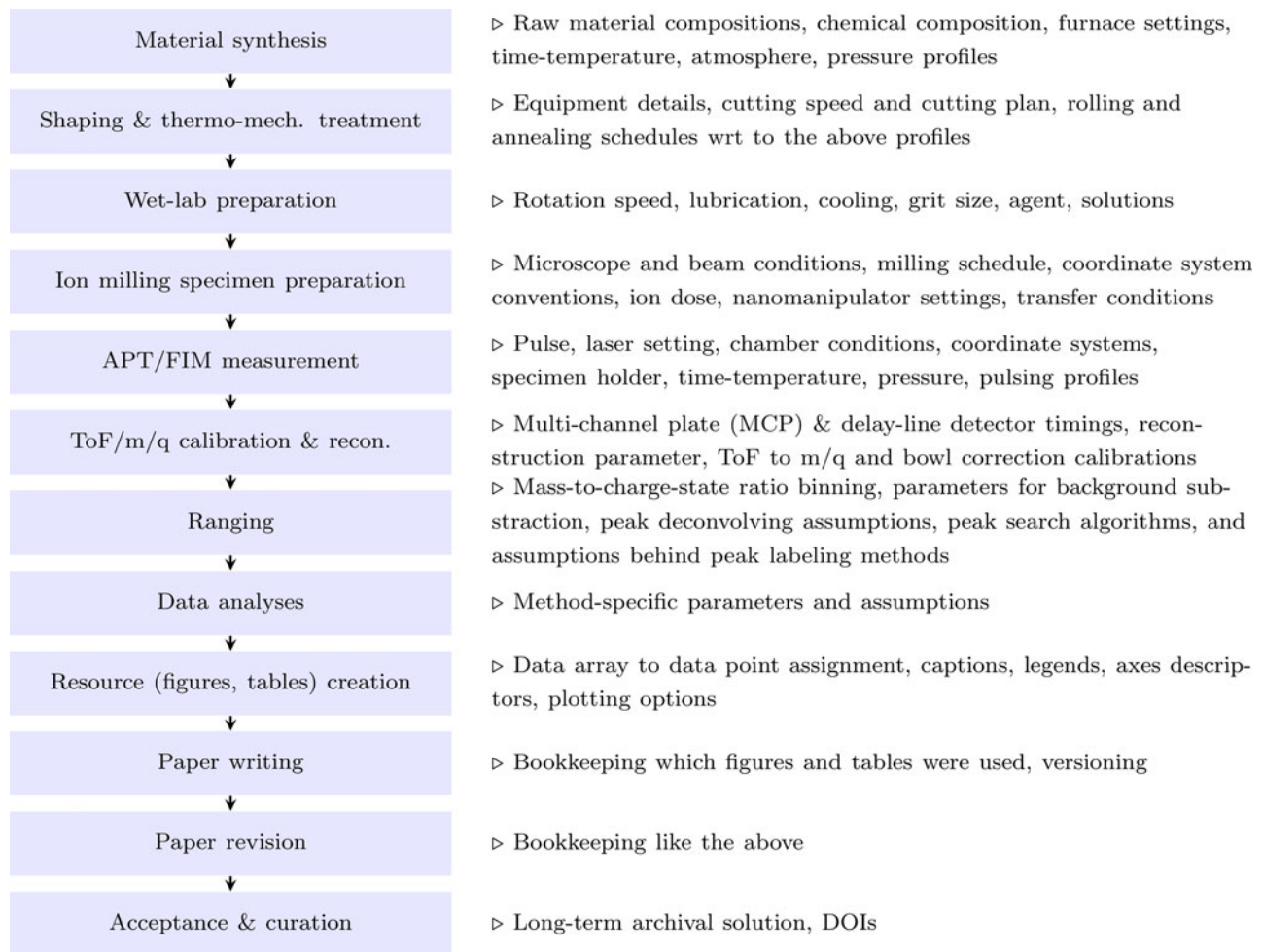
Fig. 1. To the left: Key steps of one type of scientific workflow via which many APT/FIM specimens find entry into publications. To the right, an associated (incomplete) list of exemplary (meta)data which experimentalists ideally need to keep track of during each step.
