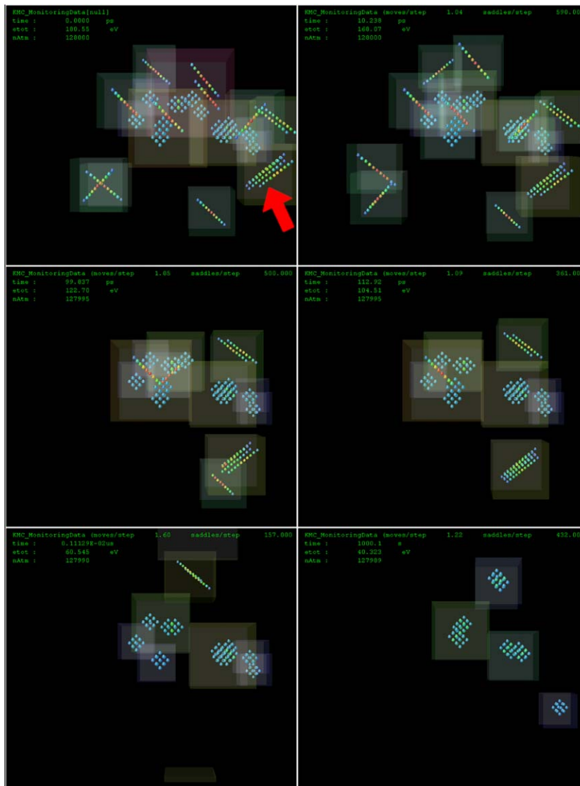
Figure 8. Snapshots from the evolution of a 20 keV irradiation damage cascade in tungsten evolving at 600 K. Reading left-to-right and top-to-bottom, the snapshots are taken at time t = 0, 10 \text{ ps}, 100 \text{ ps}, 113 \text{ ps}, 100 \text{ ns}, 1000 \text{ s} . Starting from the top left image, the cascade starts with a number of crowdions. After 100 ps three have diffused out of the simulation cell, and two more have annihilated on vacancies. At the bottom right we see a loose 4i\langle 111 \rangle interstitial cluster, indicated by a red arrow, gather a crowdion to become a 5i\langle 111 \rangle interstitial cluster. After 150 ps only two small interstitial clusters remain, and by 120 ns both have left the simulation cell. Brownian motion of the vacancies ultimately leads to accumulation into small 3- and 4-vacancy clusters. Only high energy atoms are shown, coloured from blue (+0.1 eV) through green to red (+1.5 eV). This calculation took 26 h on a single processor.
