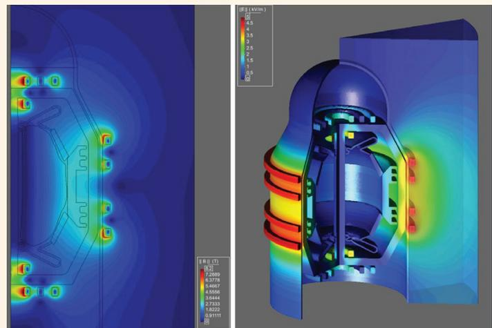
Figure 2: Magnetic flux density (left) and induced electric field (right) for the new spherical tokamak STEP (under design at UKAEA).
