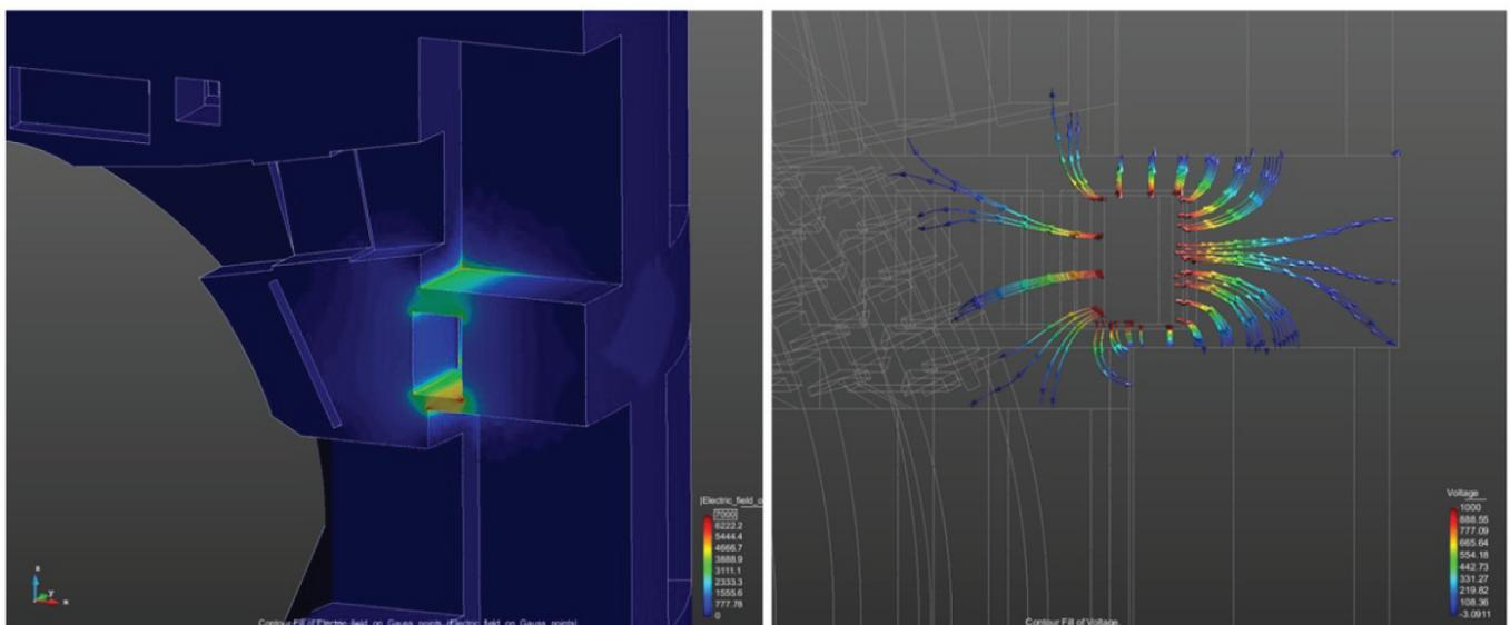
Figure 7: Detail of the electric field module (left) and electric field iso-lines (right).
