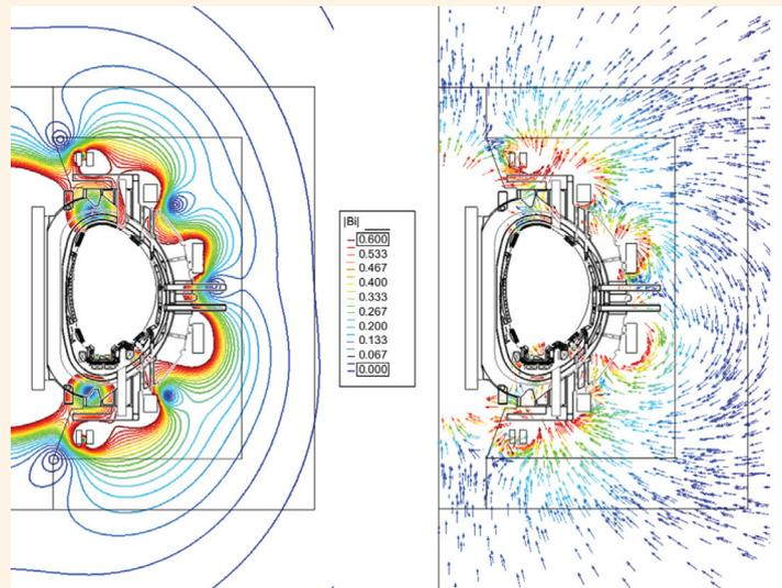
Figure 1: Magnetic flux density  $B$  before a 10 ms 6 MA plasma disruption scenario at JET.
