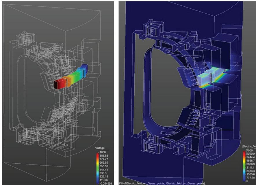
Figure 6: Voltage (left) and electric field (right) generated during a quench in ITER poloidal coil.
