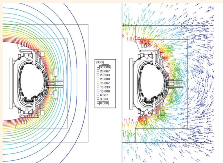
Figure 3: Time derivative of the magnetic flux density  $B$  for the 10 ms 6 MA plasma disruption scenario at JET.
