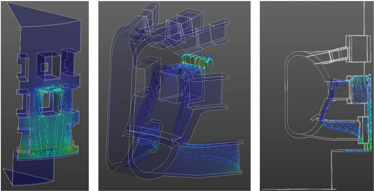
Figure 8: Electric current distribution inside the ITER cryostat and vacuum vessel.
