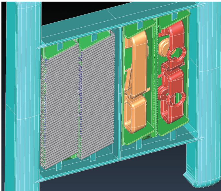
Figure 10: CAD model in GiD of the JET A2 antenna.
