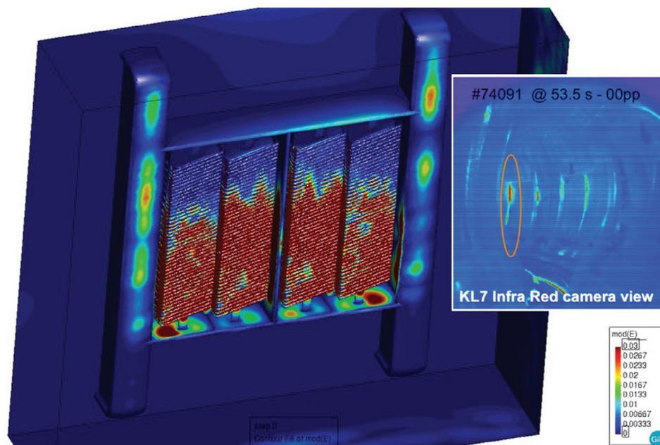
**Figure 13:** Time average of the module of the electric field calculated by ERMES and hot spots captured by the infra-red camera at JET. Work is on-going to establish the connection between the RF fields in front of the JET A2 antenna and the hot spots observed when the antenna is connected.
