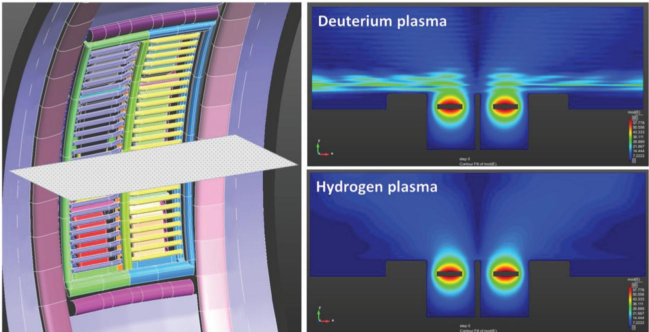
Figure 11: JET ITER-Like Antenna (ILA) and ERMES simulation of the RF fields in the marked cross section for different plasma conditions.
