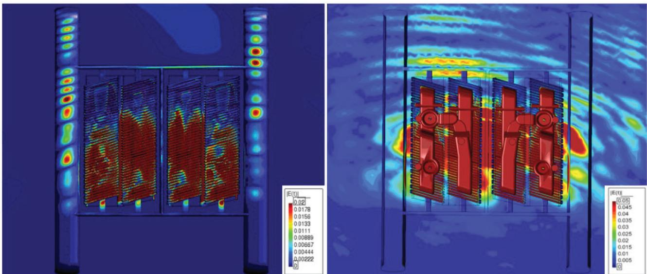
Figure 12: JET A2 antenna electric field module simulated by ERMES. Left: Front view of the antenna. Right: Back view of the antenna.
