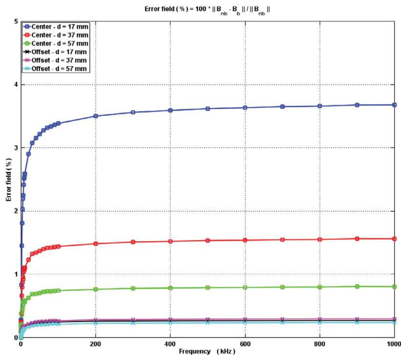
Figure 5: Error field for the two different configurations shown in Figure 4.  $B_{nb}$  refers to the magnetic flux density calculated without the frame.  $B_b$  is the magnetic flux density calculated with the frame. *Center* is the configuration at the right of Figure 4. *Offset* is the configuration at the left. *d* is the vertical distance between the coil and the bolt.
