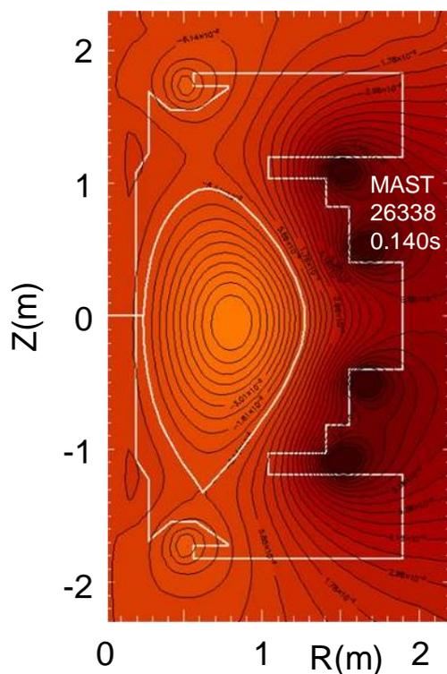
**Figure 5:** Magnetics-only equilibrium reconstruction for MAST discharge 26338 at 0.140s.
