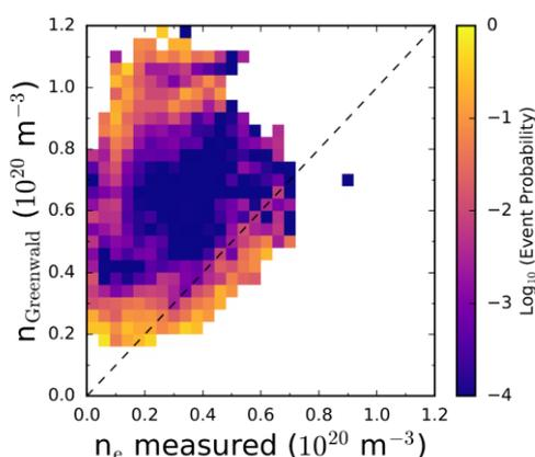
**Figure 3:** Disruptivity diagram for the MAST database in the space of measured vs. Greenwald density. Contours indicate the probability of disruption occurring in the database of plasmas in each section of parameter space.
