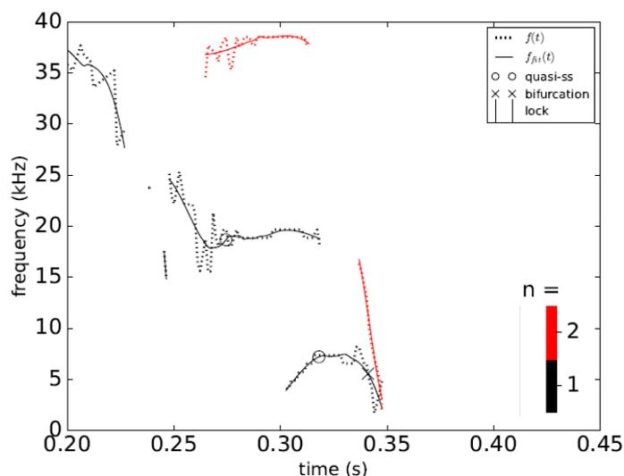
**Figure 4:** Magnetic spectrogram of MAST discharge 23447 with DECAF automatically identified events indicated, for example a quasi-steady-state period of the low frequency 2/1 neoclassical tearing mode before a bifurcation of the frequency towards locking.
