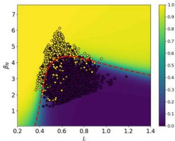
**Figure 1:**  $\beta_N$  vs  $l_i$  decision boundary for the no-wall limit on the NSTX database. The contour plot shows the probability distribution predicted by the neural network.
