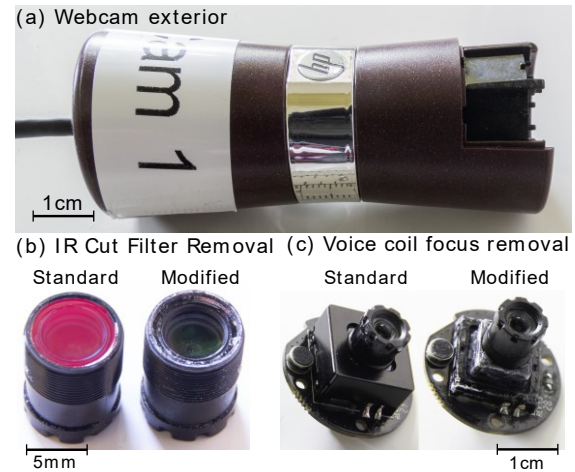
Figure 2: Photographs of (a) one of the webcams, (b) and (c) modifications made for the magnum PSI experiments.
