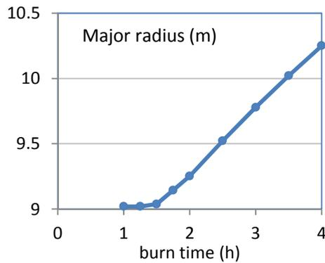
Figure 10. Major radius as a function of burn time for DEMO 1, using PROCESS, with fixed aspect ratio = 3.5. The major radius was minimised. Net electric power = 500 MW.
