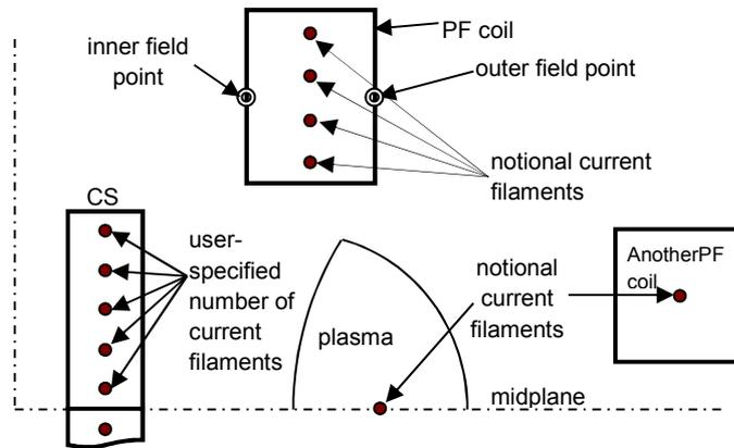
Figure 2. Model of currents used to calculate field at inner and outer radii of a PF coil
