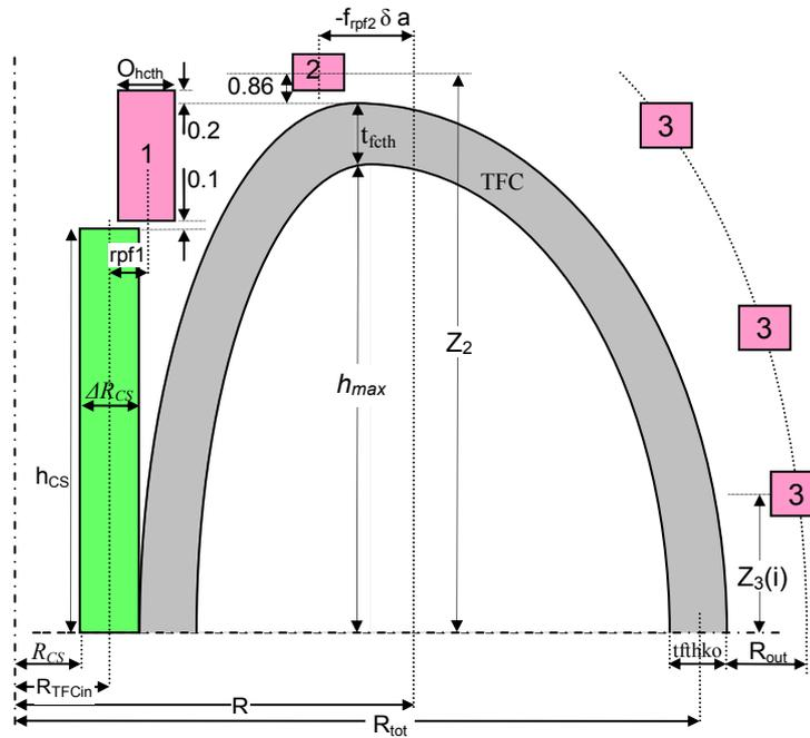
Figure 1. Geometry of CS and PF coils. The TF coil is also shown. Dimensions m.
