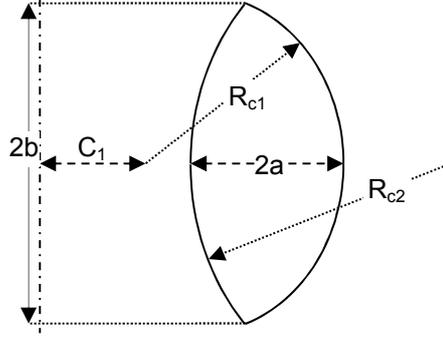
**Figure 4.** Calculation of plasma volume and surface area.
