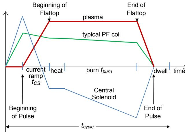
**Figure 6.** Illustration of the current waveforms and the reactor cycle.
