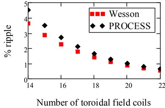
Figure 3. Ripple at the outer edge of the plasma calculated using PROCESS formula, compared to formula from (7).  $R=9$  m,  $a=2.381$  m, outer leg radius  $R_{tot} = 14.42$  m
