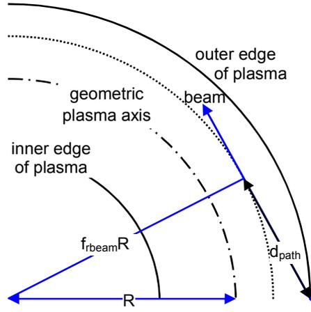
**Figure 5.** Geometry for calculating the distance travelled by the neutral beam
