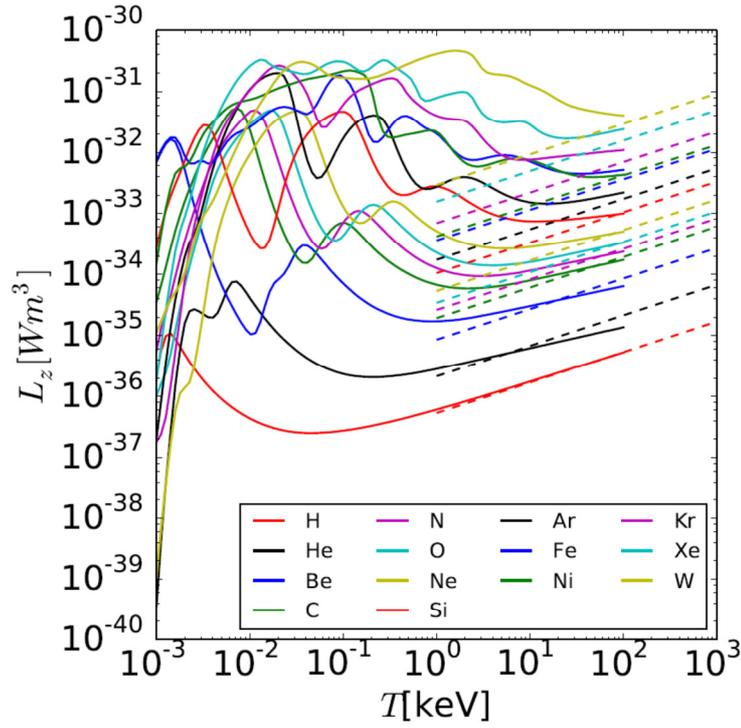
Figure 7. Radiation loss functions as a function of temperature, at  $10^{19}$  electrons  $m^{-3}$ . The lowest line is H, with the other lines in the order listed. The dashed lines show the bremsstrahlung calculated using a separate method.
