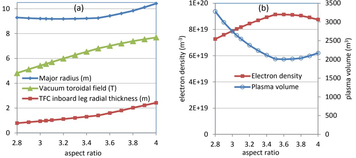
Figure 9. Parameters as a function of aspect ratio for DEMO 1, using PROCESS. The major radius was minimised. Net electric power = 500 MW, burn time = 2 hours.
