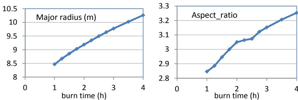
Figure 11. Parameters as a function of burn time for DEMO 1, using PROCESS. The aspect ratio and other variables were varied to minimise the major radius. Net electric power = 500 MW.
