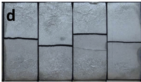
Fig. 2. Deep cracking in the armour of an ITER divertor PFC mock-up following HHF test Typical taken from [Gavali [27]].
