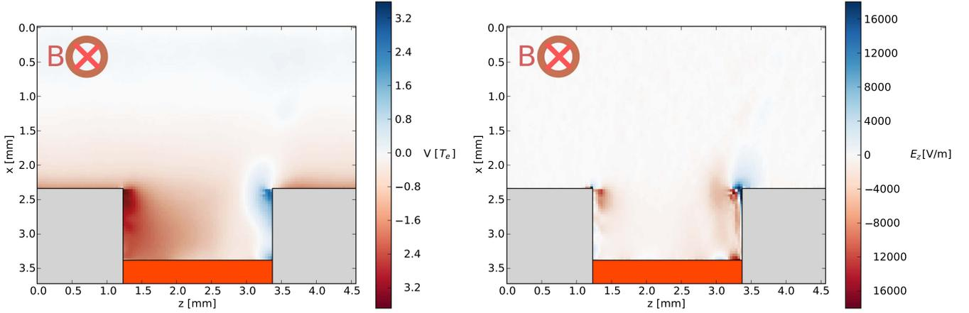
**Figure 2.** On the left—cross section of the electric potential. On the right—cross section of the resulting electric field in the  $z$  direction. Recession depth,  $h = 1.1$  mm. Particles follow the magnetic field lines into and out of the plane shown. Their orbits can take them into contact with the walls, running parallel to the magnetic field, resulting in the potential structure shown.
