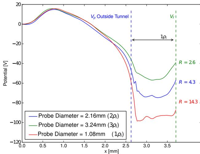
**Figure 5.** The potential structure across the simulation domain. The floating potential of the probe varies with tunnel diameter as does the value of  $R$ . The potential structure near  $x = 0$  is a result of the source sheath, an artefact of particle injection in this region.
