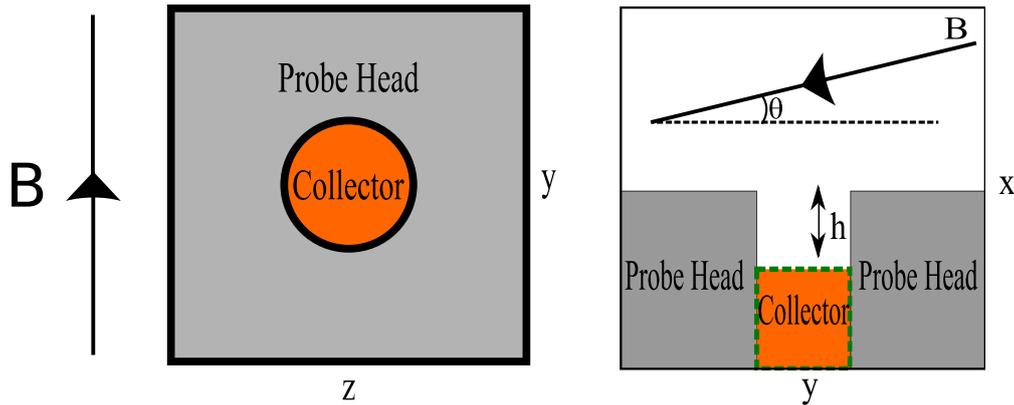
**Figure 1.** On the left—the BPP simulation domain as viewed from above looking along the  $x$ -axis. The collector sits at the bottom of the tunnel. On the right—a cross-section of the domain.  $h$  is the recession depth.
