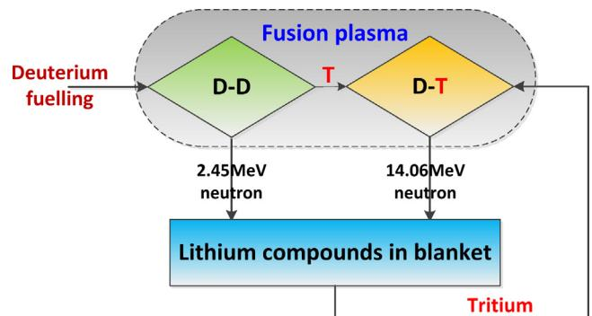
**Fig. 1.** Mechanism of fusion plasma evolvement from D-D to D-T.
