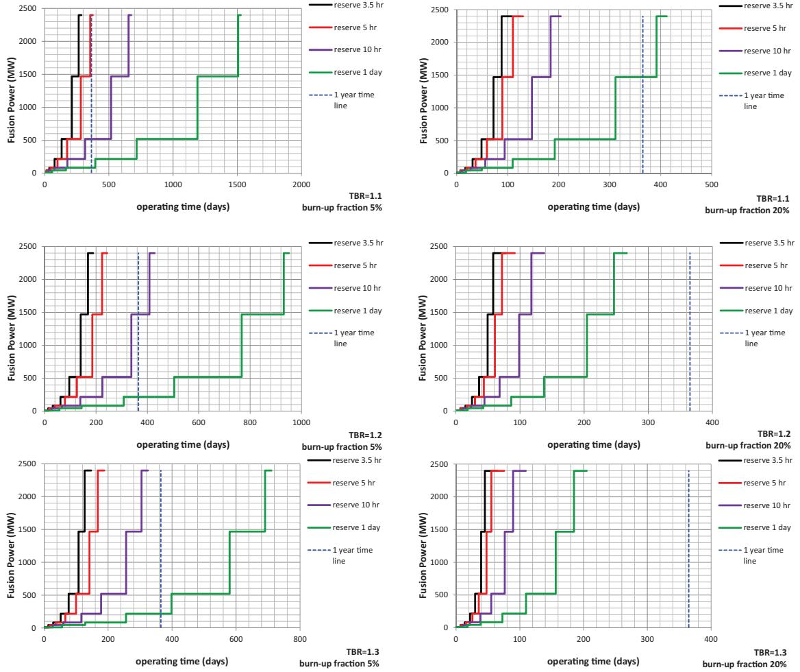
**Fig. 6.** Fusion power building up from D-D to D-T at targeted power (2.4 GW).
