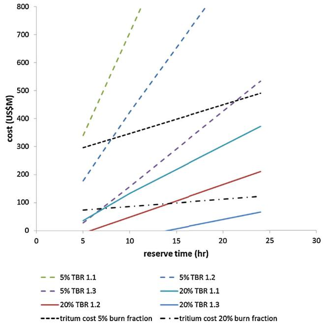
**Fig. 8.** Estimation of additional cost of tritium accumulation compared with cost of tritium required to start D-T operation for tritium accumulation off set against 6 months of the commissioning time.
